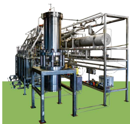
Figure 1. World's Largest SFC purification system (destined for cannabinoid purification)
